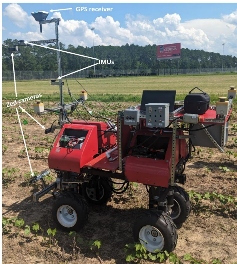
Figure 1 Front view of the rover deployed to collect video streams of cotton plants (Adapted from Thesma et al., 2024)
